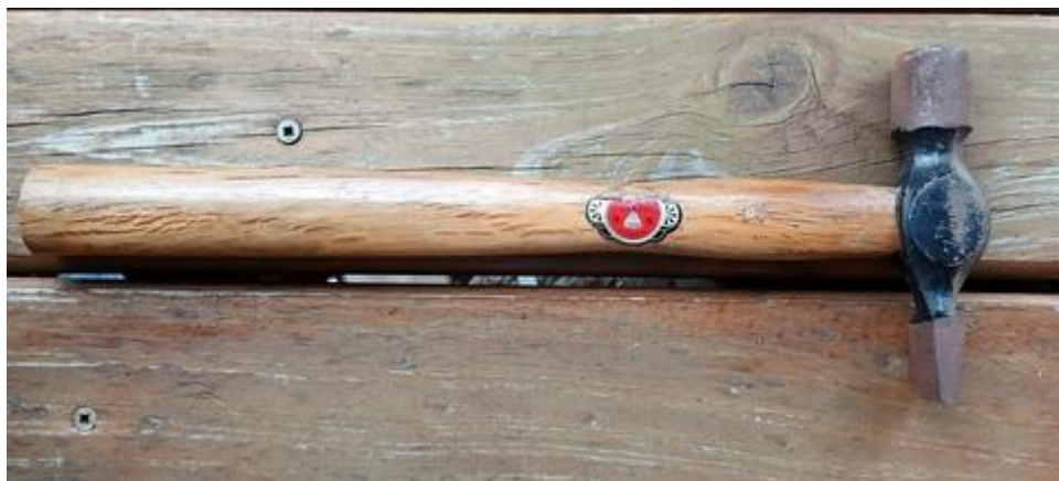
Bottom cap removal hammer!
