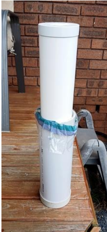
Using the inner piston to compress the plastics into the bread bag
