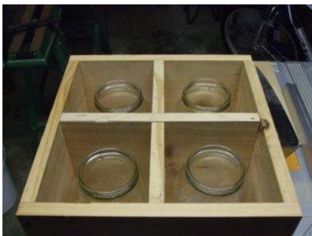
Top of box showing divider and jars in place
