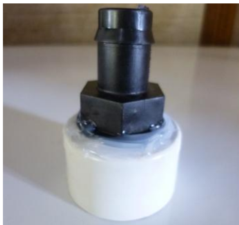
My cap with the barbed fitting siliconed on
