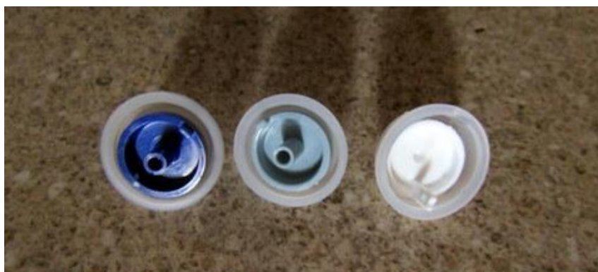
Left: original seal Centre: new replacement seal (correct) Right: New seal which look OK from the front but rear was totally different
