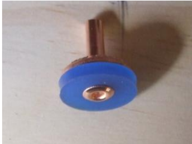
New style washer stem showing attachment rivet
