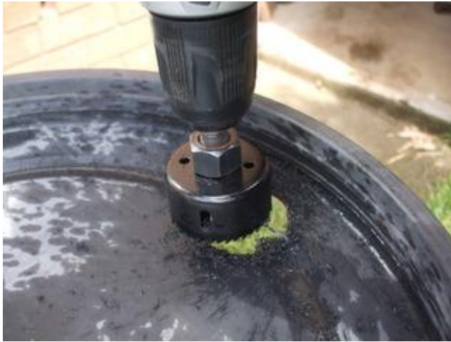
Cutting the hole in the top
