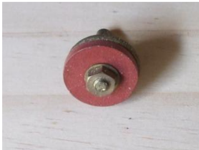
Old style washer stem showing attachment nut
