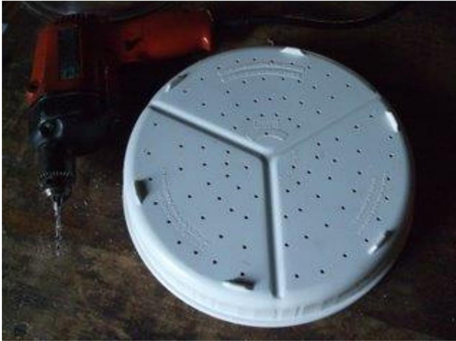
*Container with holes drilled in the bottom*
