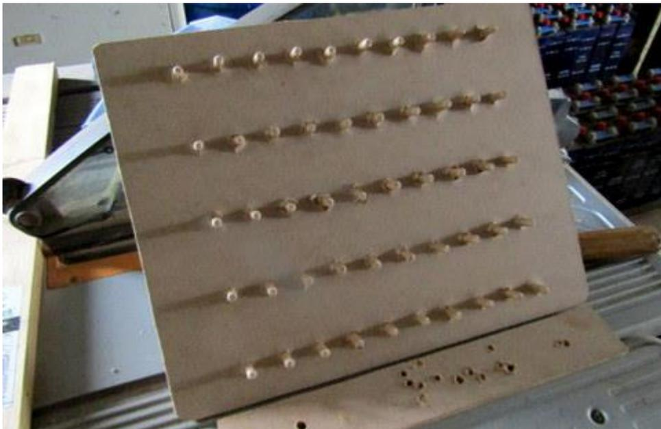
The next challenge was to work out how I would arrange it so that I could push a hole into the seed raising mix at the appropriate places, into which I would then plant a seed. For years I have had a pack of 50 fluted timber dowels (6mm in diameter x 32mm long) which were designed to be used in timber joinery but I hadn't used for anything. Only 50 you say? When I needed 100? Well I had an obvious answer, I would use the aforementioned band saw to cut them evenly in half!
