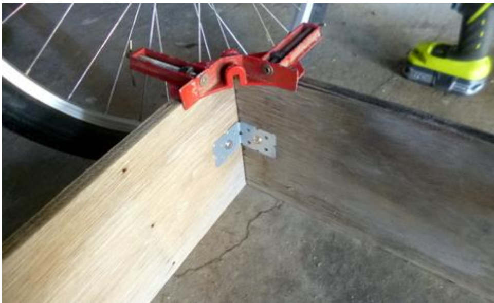
Using a picture frame vise to hold the joint steady
