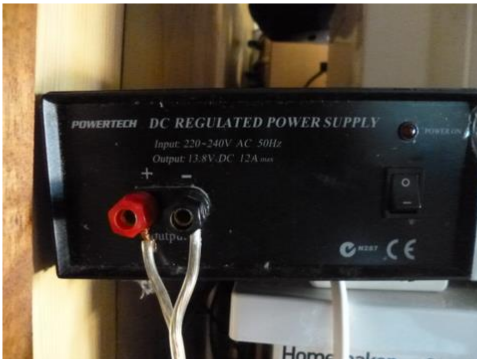
The 240vac to 12vdc power supply for the fridge
